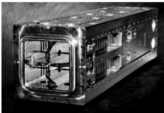
Figure 12.9 402.5 MHz four-vane RFQ that bunches and accelerates the beam from 75 keV to 2.5 MeV.
